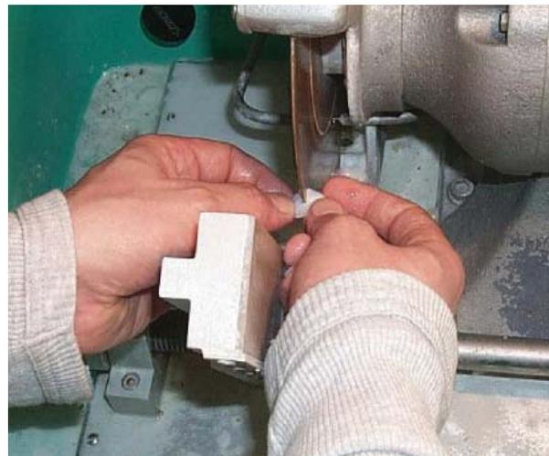
Figure 3.23. Hand cutting an otolith on the high speed thin sectioning saw.
