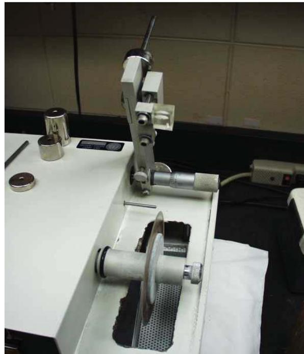
Figure 3.12. Embedded otolith mounted in low speed saw.
