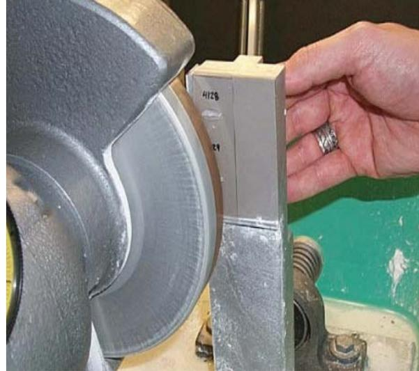
Figure 3.25. Final polishing of otolith sections using grinding arm.
