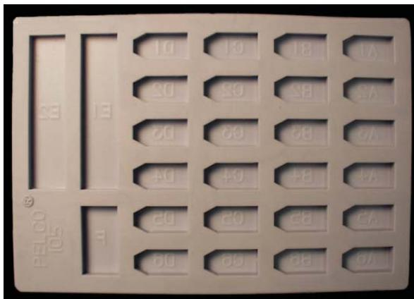
Figure 3.7 Bullet mold for embedding small or fragile otoliths.
