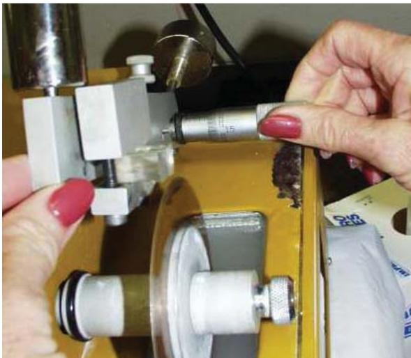
Figure 3.14. Adjusting the alignment of the block with the micrometer.
