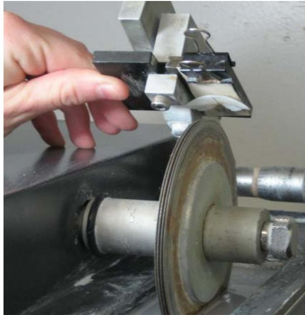
Figure 3.20 Binder clip holding cardstock in chuck preparing to be sectioned by multiple blades.
