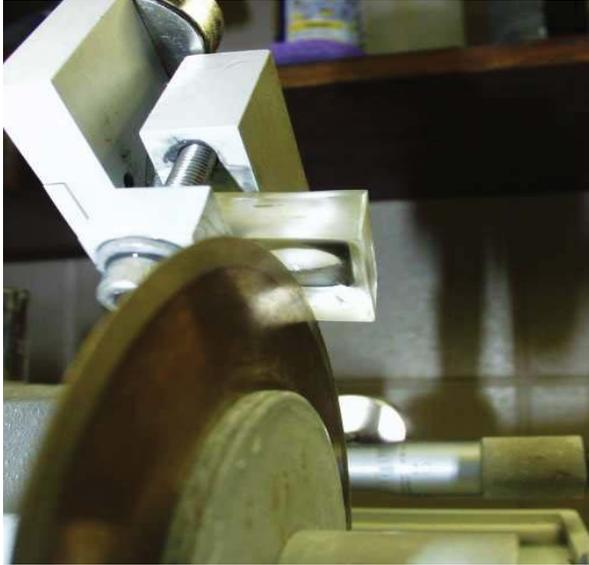
Figure 3.13 Resin block with otolith oriented against a blade at 90°.
