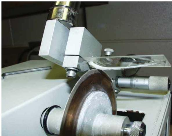
Figure 3.41. Whole spine mounted laterally to slide with thermoplastic and positioned for transverse sectioning on a low speed saw.
