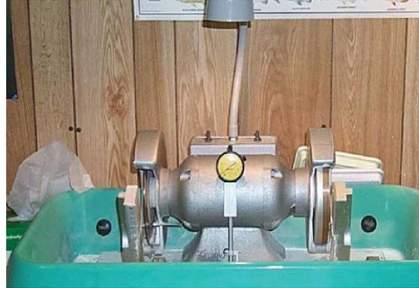
Figure 3.22. Thin section machine containing a high-concentration-diamond, continuous-rim-blade cut-off saw (left) and a precision grinder (right).
