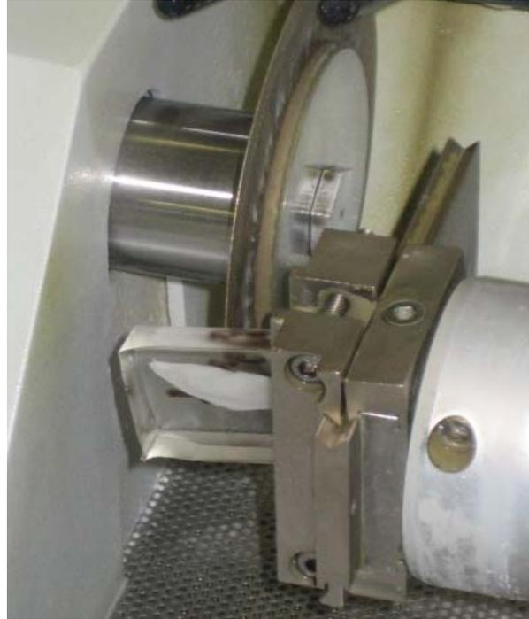
Figure 3.11. High speed wafering saw showing blade, cutting arm, coolant reservoir, and pumps with resin block ready to be sectioned.
