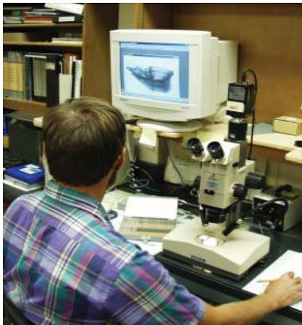
Figure 3.53. Image analysis station used to interpret an otolith section. System includes microscope, camera, computer, monitor, and interpretation software.
