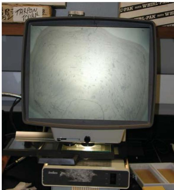
Figure 3.33 Scale impression being read on a microfiche.
