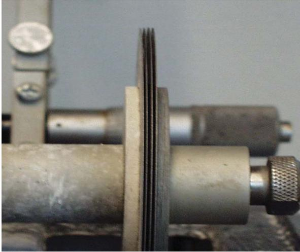
Figure 3.21 Four blades set up with spacers for production sectioning.
