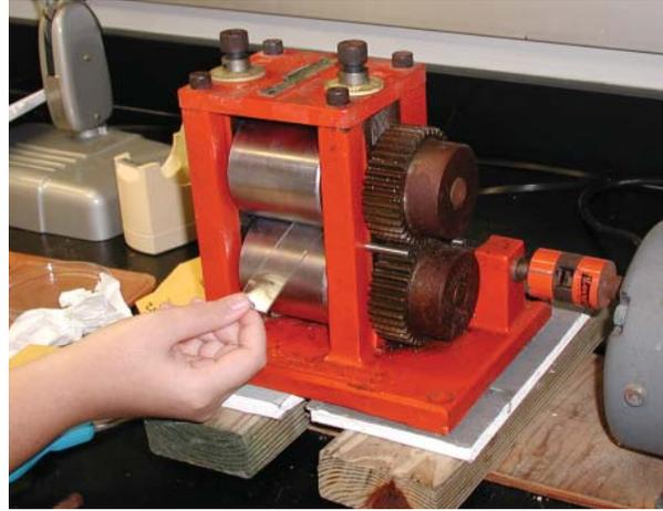
Figure 3.31 Scales on acetate passing through roller press to make impressions.
