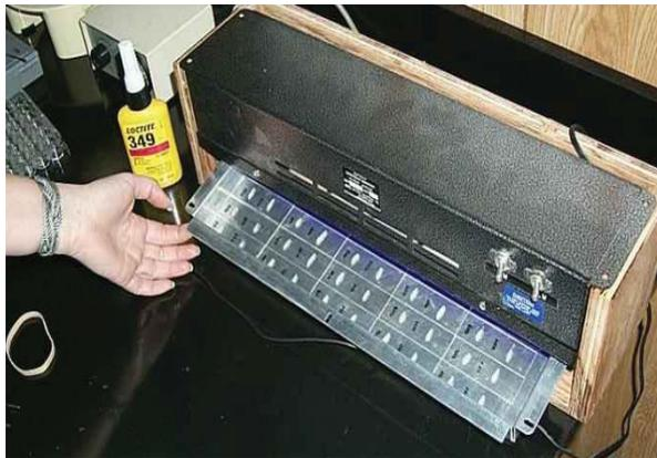
Figure 3.24. Otolith halves mounted on microscope slides with Loctite which is cured under ultraviolet (UV) light.
