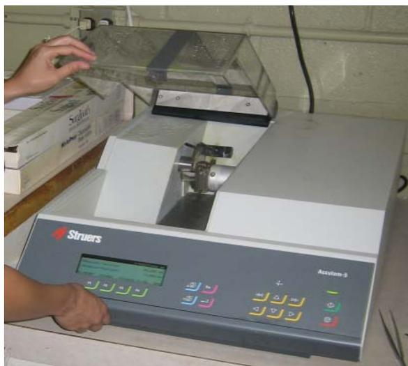
Figure 3.10. High speed wafering saw (cover opened).
