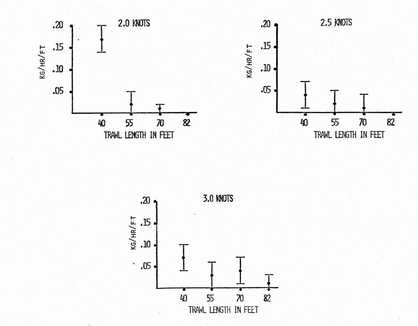
Figure 4. Mean values and associated confidence interval (95%) for total finfish at 2, 2.5, and 3 knots from <u>NOAA</u> Ship OREGON II Cruise 57. Values are expressed as kg/hr/ft of headrope and length.
