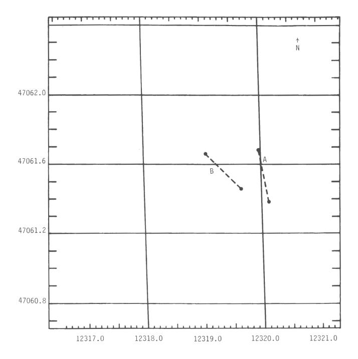
Figure 12. Targets A and B are Liberty ship hulls, plotted using data from the side scan sonar survey method.
