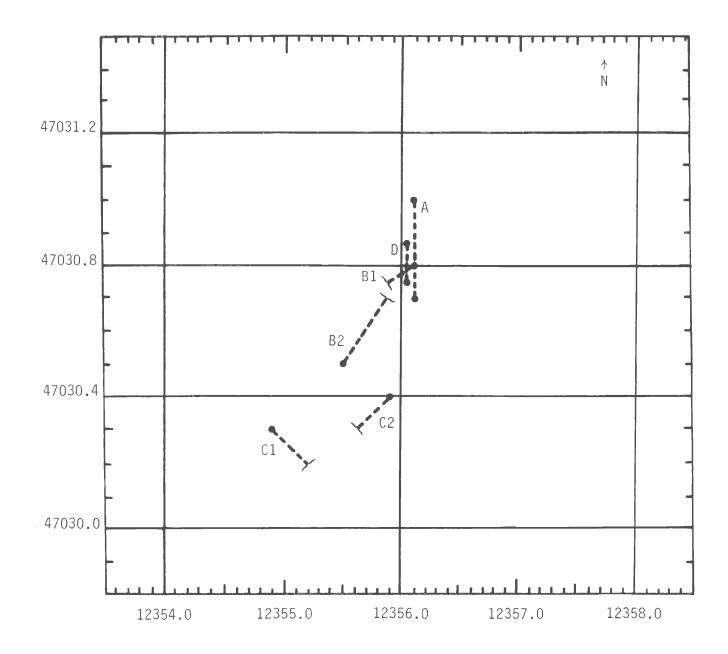
Figure 7. Target A is an intact Liberty ship hull. Targets B1, B2, C1, and C2 are each halves of Liberty ship hulls, and Target D is a barge. All targets were plotted using the SCUBA survey method.
