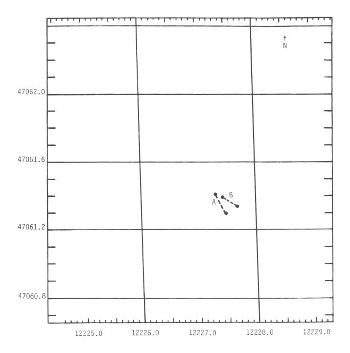
Figure 14. Targets A and B are barges at site FH-4, plotted using data from side scan sonar survey method.
