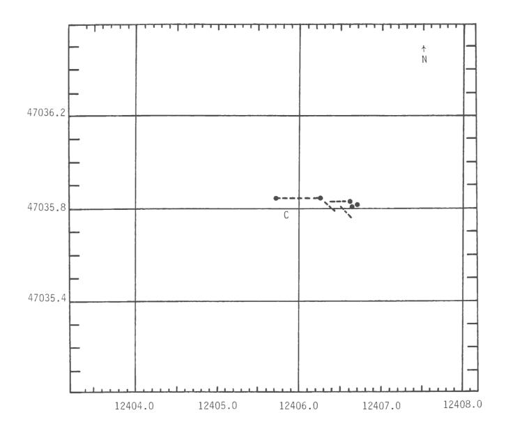
Figure 10. Target C is a barge. Material to the right of Target C was unidentifiable from the side scan sonar record. All material were plotted using data from the side scan sonar survey method.
