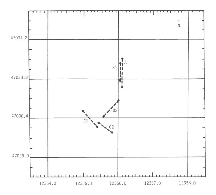
Figure 19. Target A is an intact Liberty ship hull. Target B1 is a barge which was misidentified as half of a Liberty ship hull. Targets B2, C1, and C2 are halves of Liberty ship hulls. All materials were plotted at site FH-6 using data from the side scan sonar survey method.
