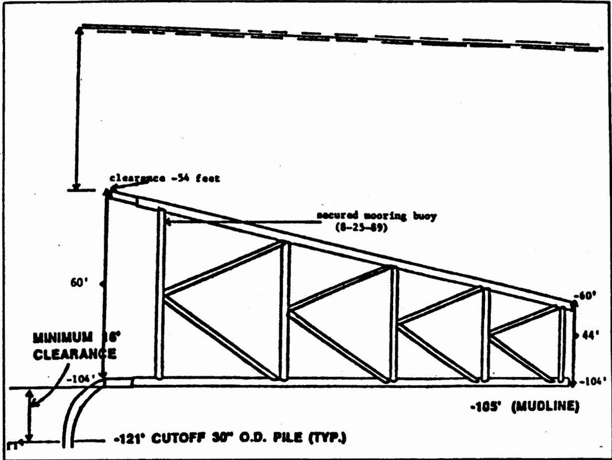
Figure 3. Schematic of sunken platform (and now artificial reef) at South Timbalier Block 86 Platform A (86-A) as viewed from above (courtesy of ODECO Oil and Gas Co.).
