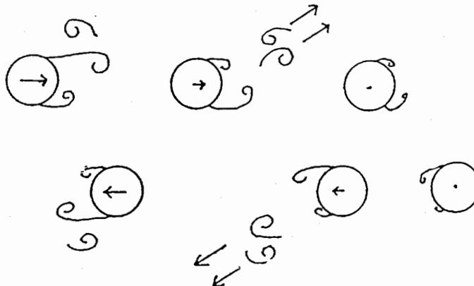
Figure 5. Schematic of flow separation for various Kuelegan Numbers (Teng, 1986). Arrows within cylinder depicts the flow direction driven by the wave passage.
