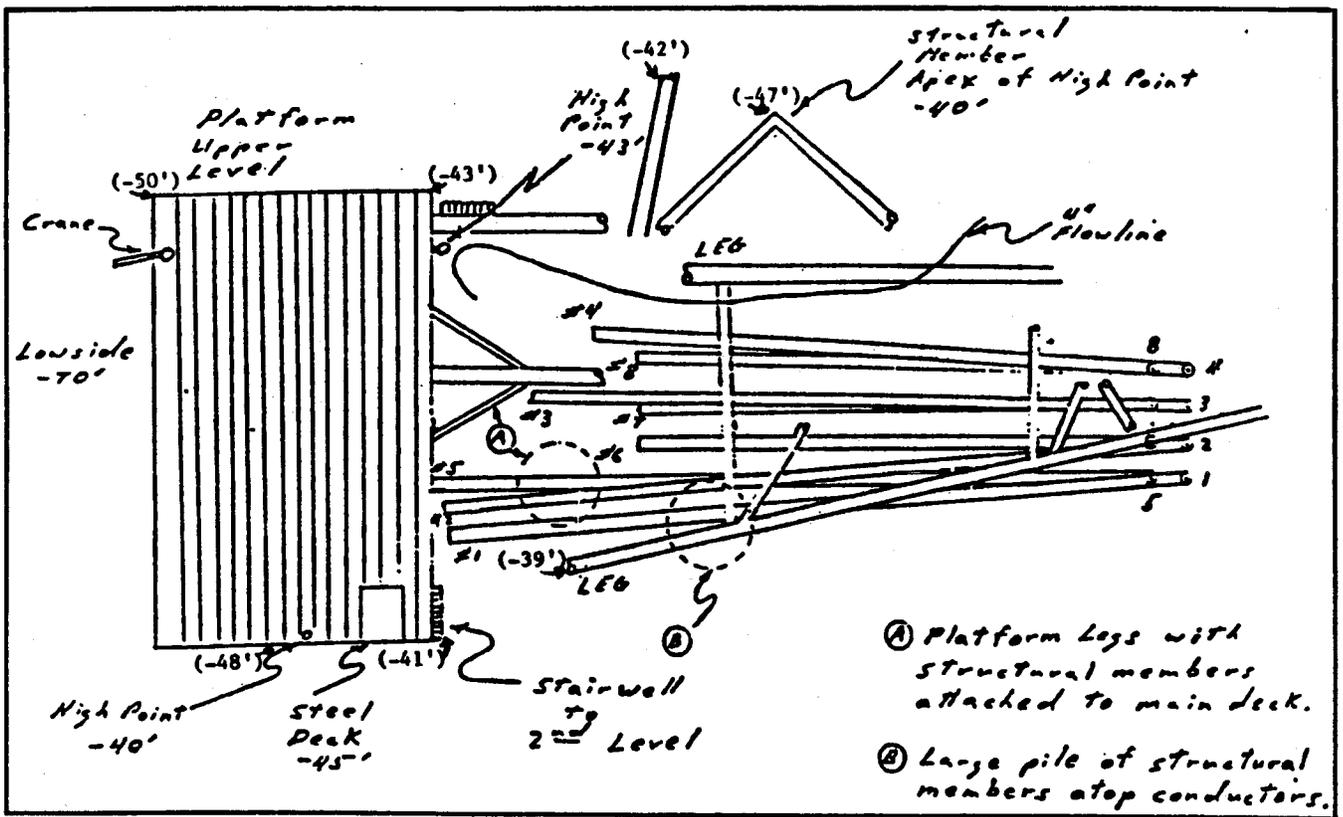
Figure 4. Schematic of toppled platform (and now artificial reef) South Timbalier Block 128 Platform A (128-A) as viewed from the side (courtesy of Chevron U.S.A., Inc.).
