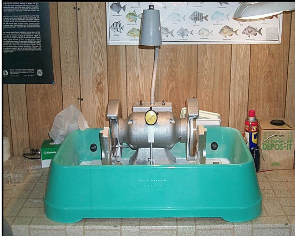
Figure 3.17. Thin section machine containing a high-concentration-diamond, continuous-rim-blade cut-off saw (left) and a precision grinder (right).
