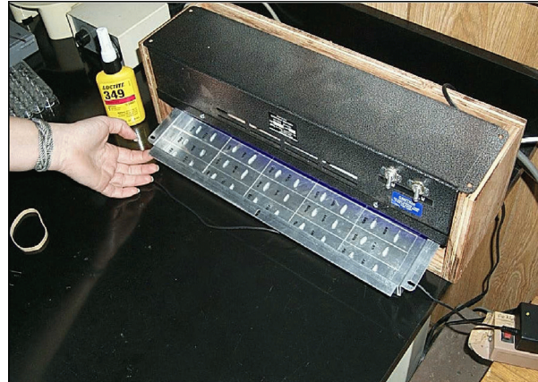
Figure 3.19. Otolith halves mounted on microscope slides with Loctite which is cured under ultraviolet (UV) light.
