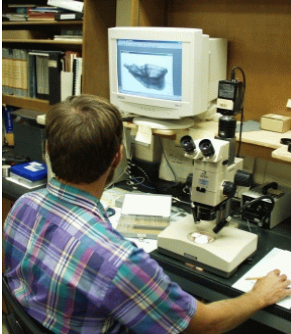
Figure 3.45. Image analysis station used to interpret an otolith section. System includes microscope, camera, computer, monitor, and interpretation software.
