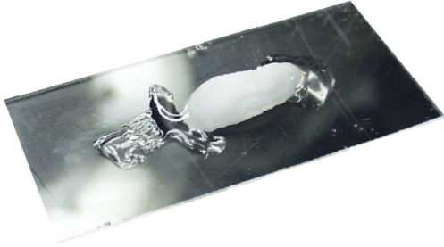
Figure 3.8. Otolith mounted to a glass slide using thermoplastic on each end. The central portion of the otolith must remain clear of adhesive.
