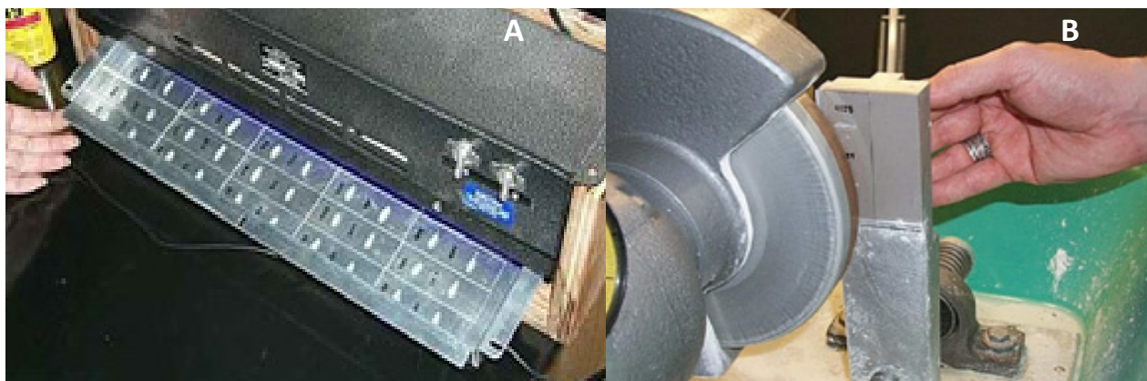
Figure 3.34 A) Otolith halves mounted on microscope slides with Loctite which is cured under ultraviolet (UV). B) Final polishing of otolith sections using grinding arm.
