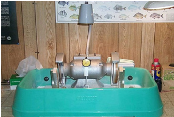
Figure 3.32 Thin section machine containing a high-concentration-diamond, continuous-rim blade cut-off saw (left) and a precision grinder (right).
