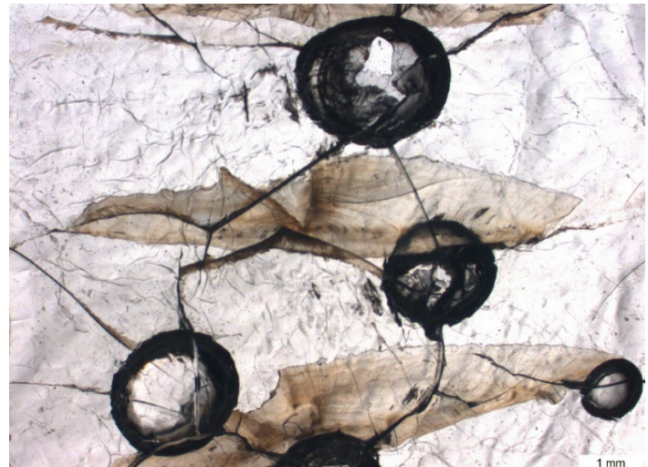
Figure 2.5 Otolith section that has been covered with Loctite® and has cracked over time.
