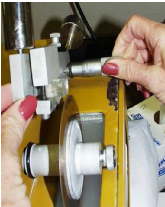
Figure 3.25 Alignment of the block to the blade is made by adjusting the micrometer.
