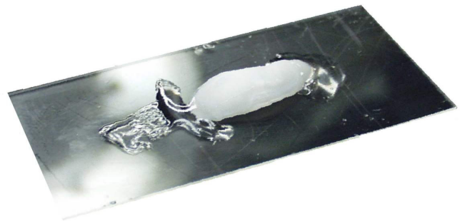
Figure 3.20 Otolith mounted to a glass slide using thermoplastic on each end. The central portion of the otolith must remain clear of adhesive.
