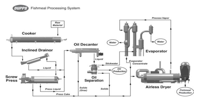
**Figure 7.1** The processing of raw menhaden through a modern reduction plant (diagram courtesy Dupps 2014).
